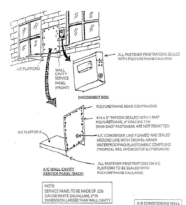
CAVITY SERVICE PANEL / FASTENER DETAIL REQUIREMENT
